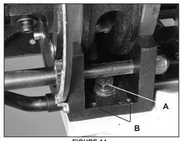
**FIGURE 14**Photo of the micro adjusting screws shown with table angled for clarity.
