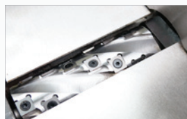
Helical Cutterhead with Inserts Cuts Smooth and Fast
