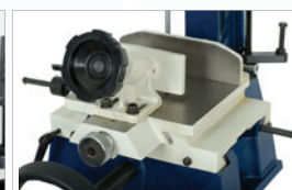
X-Y Table moves Left-to-Right & Front-to-Back
