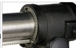
Degree Labels for Quick Setting of Head or Table Angles
