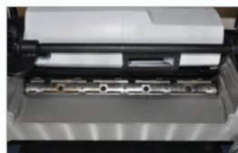
Helical-Style Cutterhead Gives Easy Blade Access
