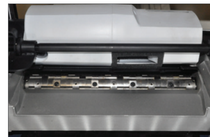
EASY ACCESS TO CUTTERHEAD TO CHANGE INSERT BLADES
