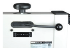
QUICK-RELEASE BLADE TENSION LEVER
