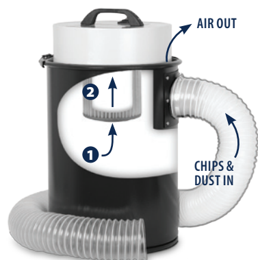
TWO STAGE FILTRATION WITH CARTRIDGE & FILTER BAG
