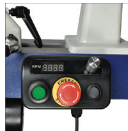
CONTROL BOX WITH MAGNETIC BACK ATTACHES TO LATHE
