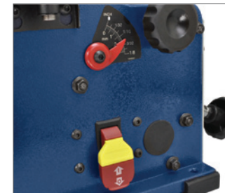
DEPTH SCALE AND SAFETY ON/OFF SWITCH
